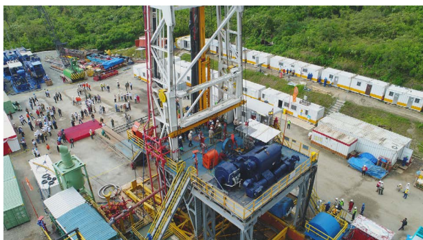
Production well drilling at the Muara Laboh power station (left) and a panoramic view of the entire site
