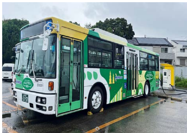
Retrofitted EV bus assembled in Japan (operating in Fukuoka City from June 2023)
